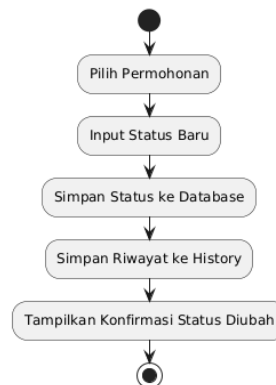
Gambar 11. Activity Diagram Ubah Status Permohonan
