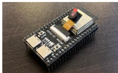
Gambar 2. ESP32-S3 Cam OV2640
